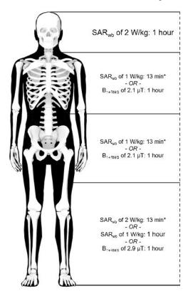
Landmark restrictions for time and exposure conditions for the  $\mbox{SpF}^{\circ}$  PLUS-Mini in 3T scanners.
