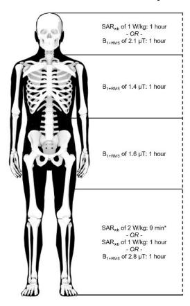
Landmark restrictions for time and exposure conditions from the  $\mbox{SpF}^{\circ}$  XL-IIb in 3T scanners.
